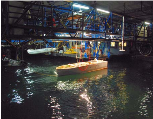
Fig. 27 Model and the towing carriage.
