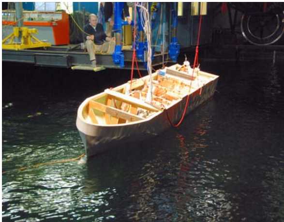
Fig. 29 The model was kept in beam seas with occasional control by two lines connected to the bow and stern of the model, if necessary.
