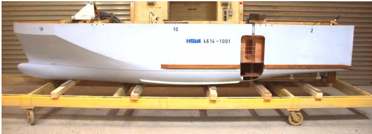
Fig. 25 The model HSVA No. 4614 of the ship EMSA1 with the opening of the Damage Case 1.
