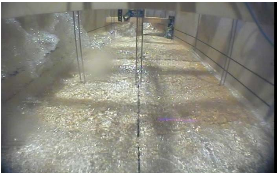
Fig. 72 One of the selected frames from a video recording of the measurement no. 35. The frame shows water sloshing over 6 m high against the port side wall.
