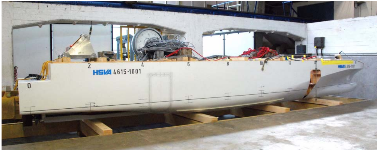
Fig. 49 The model HSVA No. 4615 of the ship EMSA2/EMSA2MOD with the opening of the Damage Case 4 at the ship side. The closed opening for the Damage Case 1 can also be seen between the stations 4 and 6.
