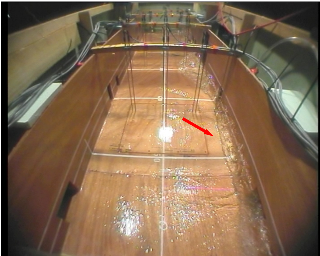
Fig. 63 Water sloshes against the damaged side wall. The water elevation at the wall exceeds the first white line at 1 m height.
