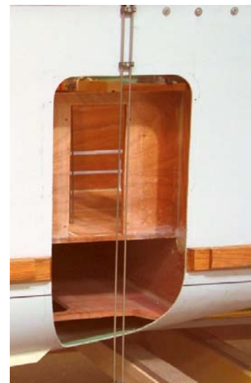
Fig. 26 The damage opening of the Damage Case 1.
