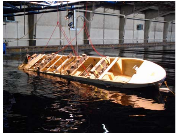
Fig. 54 The list grows further and a full capsizing of the model is avoided only with the help of the red "preventer" lines.
